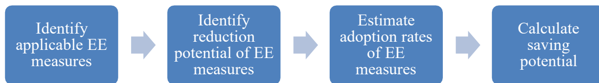
Figure 40. Method to quantify energy-saving and emission reductions potential
